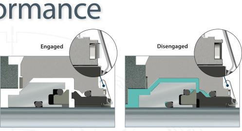
**Before Installation** The spring lifter is engaged and retracts the stationary face, providing ample space between the seal faces for ease of installation.
