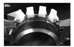
Spring lifter clips installed in gland halves.
