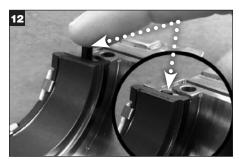
To prevent seal leakage, ensure that the stationary face O-Ring ends are flush with but not below the stationary face splits. Carefully push on O-Ring ends if they protrude past the face splits. Preparation complete; go to **Seal Installation**
