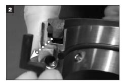
Remove used rotary holder gaskets.
