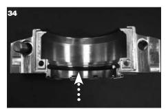
Apply a thin film of grease to the stationary face O-Ring halves and install in gland halves; Ensure that O-Ring splits are protruding evenly on both
