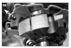
Carefully remove the gland installation tool, taking care not to dislodge the gland stuffing box gasket. Retain the gland installation tool for future use.
