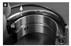
Remove used rotary face O-Ring halves.
