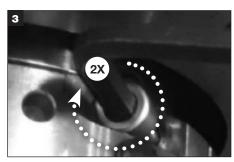
Use hex wrench and alternately tighten holder cap screws to finger-tightness to allow holder to slide along the shaft. Caution: Care should be taken not to rotate the rotary holder on the shaft.
