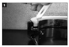
Equipment shaft should be cleaned and greased prior to rotary holder installation. Apply supplied grease only to face splits. Do not apply grease to o-ring ends. **Caution:** Dirt particles on seal face splits may cause leakage. The rotary holder should not be rotated on the shaft during Steps 2 through 4 as it may lead to shaft leakage and/ or face damage.
