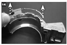
Remove spring lifter halves from gland halves.
