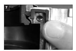
Ensure that the gland gaskets are lubricated and seated in their grooves.
