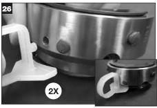
Install installation spacers on outside diameter of holder halves.
