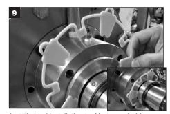
Install gland installation tool between holder assembly and stuffing box face.
