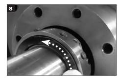
Clean rotary face with supplied cleaning wipe, ensuring there is no debris at splits. **Caution:** Do not push on seal face - it may cause the seal face to misalign resulting in seal leakage.
