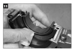
Clean stationary face with cleaning wipe, ensuring that there is no debris at splits.
