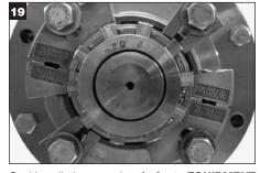
Seal installation complete (refer to EQUIPMENT STARTUP). Note: Four bolt configuration is shown. (refer to Figure 4 - Mounting Configurations for other bolt quantities).
