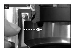
Remove used gland gaskets from gland grooves.
