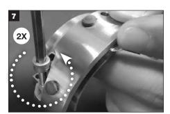
Remove used holder cap screws from holder halves.
