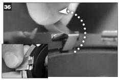
Install spring retainers in gland halves, holding the stationary seal ring half in the gland.
