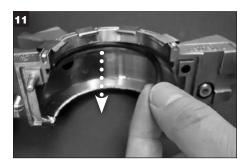
Remove used stationary face O-Ring.
