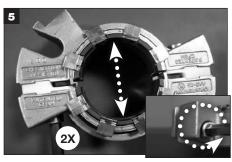
Disengage gland cap screws and separate gland halves.
