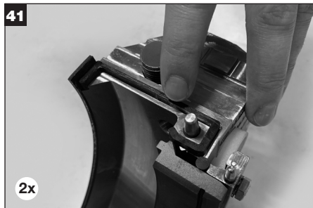
Apply a thin film of grease to gland gaskets and install in grooves of gland halves. Note: Gland gaskets must be installed on gland end where stuffing box face gasket protrudes.
