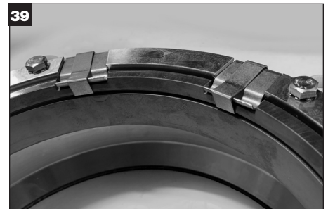
Spring retainer installed.
