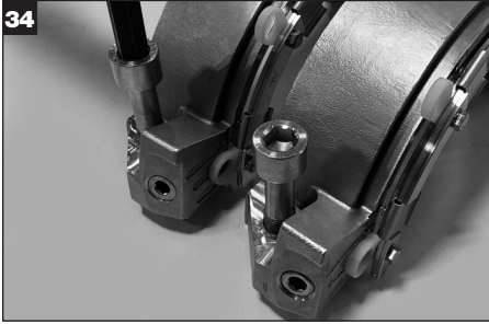
Install gland cap screws in gland halves (2x). Note: Gland cap screws are installed in one end of each gland half, in the ends away from the mounting bolt slot.
