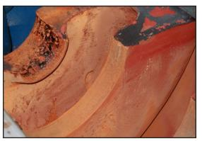
Eroded and corroded pump volute
