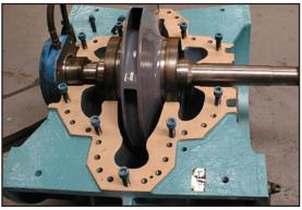
ARC-coated surfaces - casing and impellor
