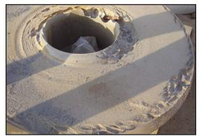
Damaged wear plate at 22 days
