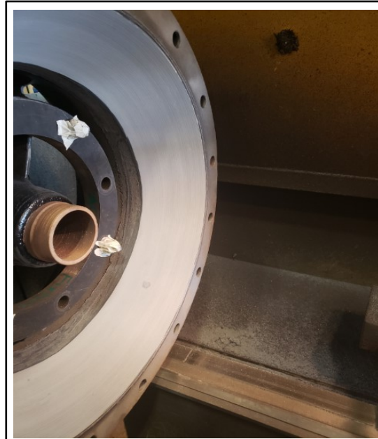
Suction bell being machined after ARC 858 was applied.
