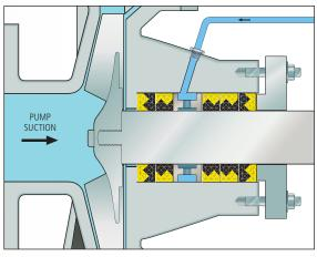
FIGURE 2 – Solids Resistance and Anti-Extrusion
