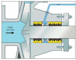
FIGURE 1 – All Rings Oriented for Sealing
