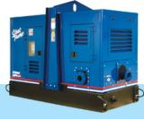
The modular design, featured on several PA Series® pump models, enables the addition/ removal of a lightweight, aluminum, acoustically-treated enclosure to the standard fuel base. The enclosure provides excellent corrosion resistance and offers a significant reduction in sound levels (68 dBA at 23').
