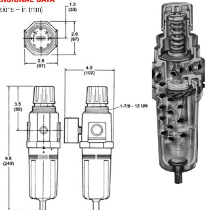
**CAUTION:** Outlet pressure adjustment ranges are not minimum or maximum outlet pressure limits. Regulators can be adjusted to zero psig secondary pressure and, generally, to pressures in excess of those specified. The use of these regulators to control pressures outside of the specified ranges is not recommended.
