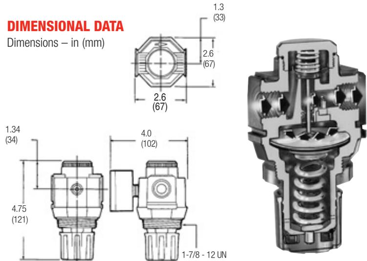
**CAUTION:** Outlet pressure adjustment ranges are not minimum or maximum outlet pressure limits. Regulators can be adjusted to zero psig secondary pressure and, generally, to pressures in excess of those specified. The use of these regulators to control pressures outside of the specified ranges is not recommended.
