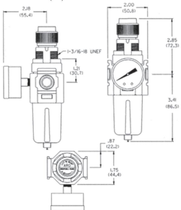
*CAUTION: Outlet pressure adjustment ranges are not minimum or maximum outlet pressure limits. Regulators can be adjusted to zero psig secondary pressure and, generally, to pressures in excess of those specified. The use of these regulators to control pressures outside of the specified ranges is not recommended.*
