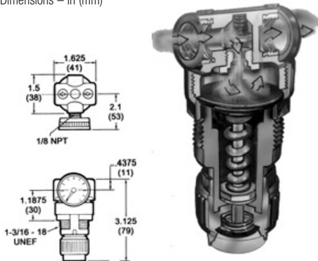
**CAUTION:** Outlet pressure adjustment ranges are not minimum or maximum outlet pressure limits. Regulators can be adjusted to zero psig secondary pressure and, generally, to pressures in excess of those specified. The use of these regulators to control pressures outside of the specified ranges is not recommended.
