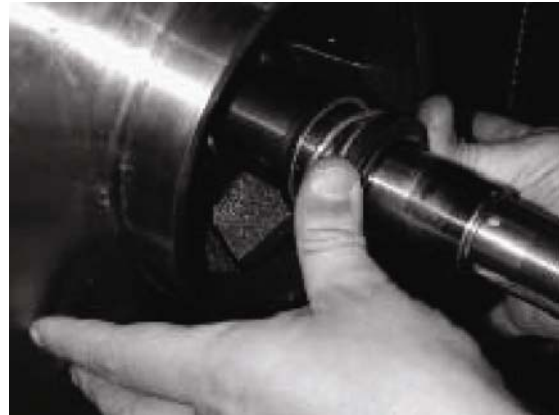
Figure 25: Installing Mechanical Seal Head
