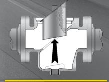
When the basket requires cleaning, simply vent system pressure, remove the lid and withdraw the basket from the top. Foreign matter contained in the basket will not drop back into the system.
