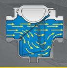
The inclined position of the strainer basket adjacent to the porting allows for smooth flow patterns.
