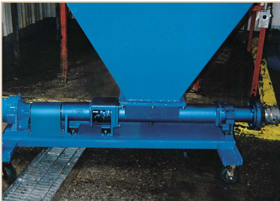
Transferring dewatered filter cake at 20 gpm and 20 psig.
