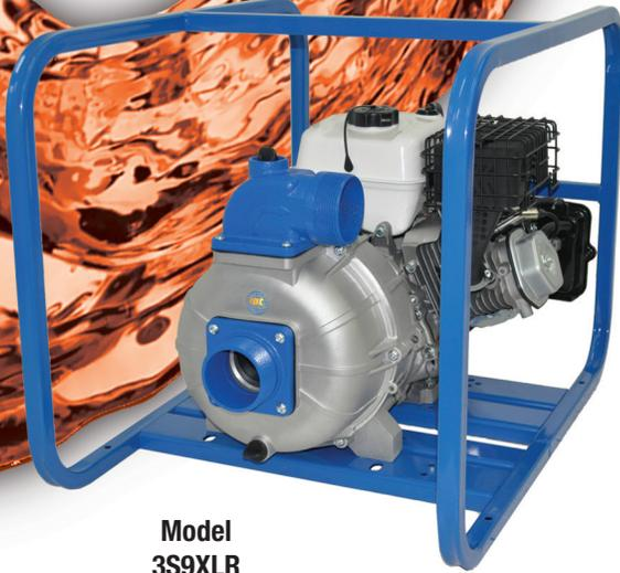
IPT Portable High Volume, Self-priming Centrifugal Trash pumps include easy cleanout with replaceable cast iron impeller and volute that resist abrasion/wear. Pumps are designed to handle liquids with solids content or dissolved solids and debris. All pumps feature aluminum housing, cast iron wearparts, built-in check valve, suction strainer and heavy duty steel roll frame. Heavy duty cast iron flanges with male NPT threads that rotates in 90° increments. Easy access fill plug on discharge port.
