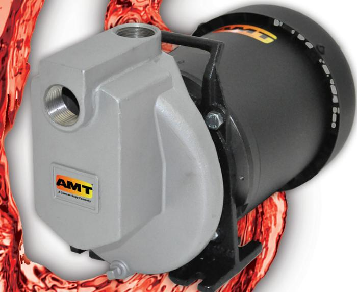
AMT 300 Series Investment Cast Stainless Steel Transfer pumps are designed to handle liquids and chemicals with specific gravities to 1.6. The pumps are particularly well suited to applications involving perchloroethylene (PCE) and are recommended for use with non-flammable liquids. Pumps are designed to handle liquids with solids content or dissolved solids and debris.
