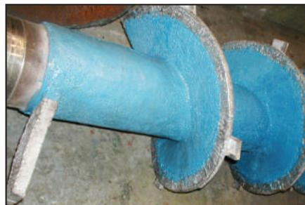
ARC MX1 applied and tips welded.
