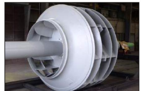
Dynamically balanced ARC S7 AR coated fan.
