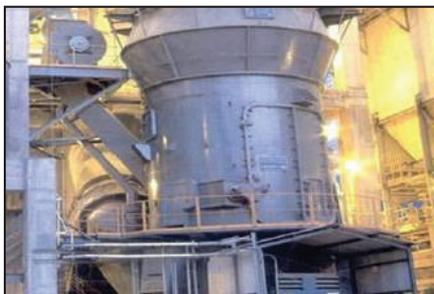
MPS Coal Pulverizer.
