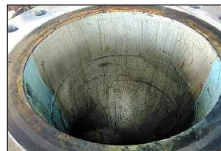
ARC S5 prevented corrosion and scale formation after 27 months.
