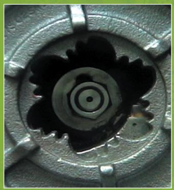
Shredder pumps can handle most unintended items that occasionally enter the waste stream.
