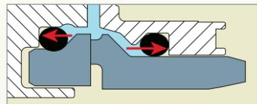
Under pressure conditions, the seal ring halves are forced together.
