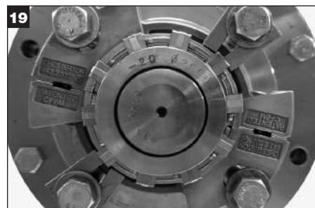
19 Seal installation complete (refer to EQUIPMENT STARTUP). Note: Four bolt configuration is shown. (refer to Figure 4 - Mounting Configurations for other bolt quantities).
