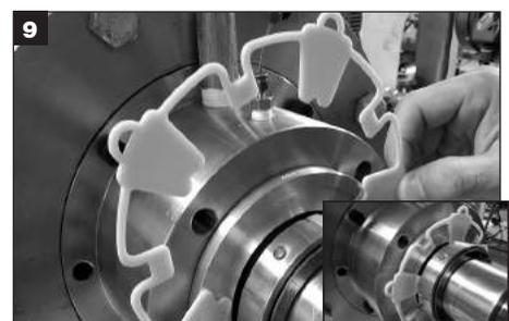
Install gland installation tool between holder assembly and stuffing box face.
