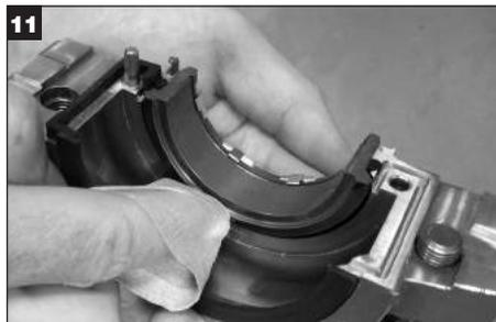
11 Clean stationary face with cleaning wipe, ensuring that there is no debris at splits.
