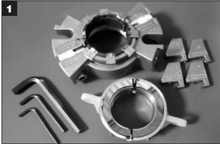
Remove seal from packaging and place on clean work surface. Ensure installation spacers are seated on outside diameter of rotary holder halves. **Important: DO NOT** glue any O-Rings, holder or gland half gaskets!
