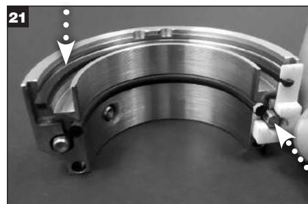
Install rotary holder shipping spacers in rotary holder halves to hold the rotary face O-Ring in place.
