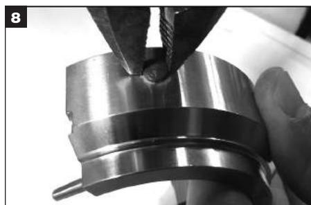
8 Remove used centering buttons from outside diameter of rotary holder.
