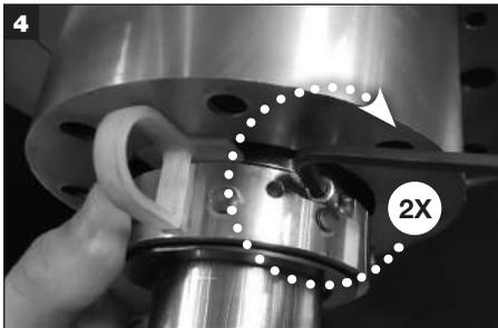
Push holder assembly so that plastic installation spacers contact the stuffing box face. **Use hex wrench and alternately tighten holder cap screws** (Refer to Table 3 - Holder Cap screw Torque Values). Ensure gaps at holder splits are equal on both sides (see Figure 5). **Caution: DO NOT** push directly on seal face.
