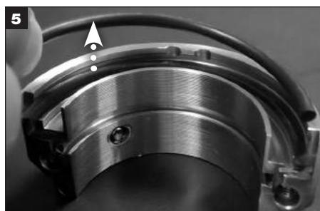
5 Remove used rotary face O-Ring halves.
