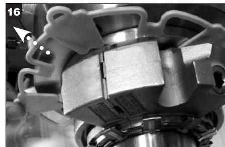
16 Carefully remove the gland installation tool, taking care not to dislodge the gland stuffing box gasket. Retain the gland installation tool for future use.
