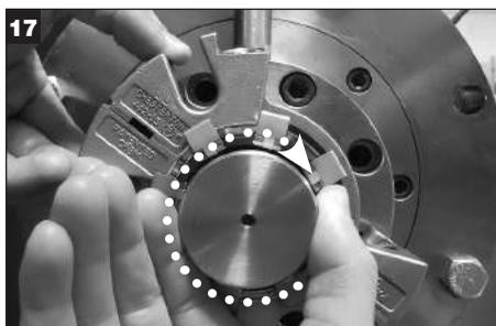
17 If possible rotate gland together with shaft when aligning gland bolt slots with the stuffing box bolt holes (refer to step 12).
