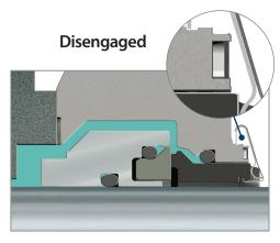
After installation, the spring lifter automatically disengages while the gland halves are assembled, initiating spring force between the two seal faces.
