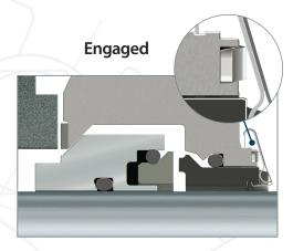
The spring lifter is engaged and retracts the stationary face, providing ample space between the seal faces for ease of installation.
