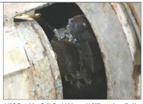
442C Cartridge Split Seal 114 mm (4.50") was installed in less than two hours.
