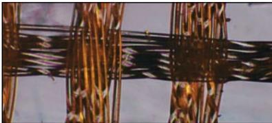
**Multifilament Mesh** is a woven fabric where each strand consists of many smaller diameter threads.
