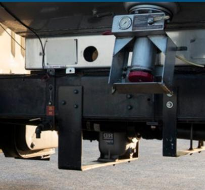
Gorman-Rupp self-priming centrifugal Power Take-Off Pumps are ideal for handling aircraft fuels, fuel oil, gasoline and other petroleum derivatives.
