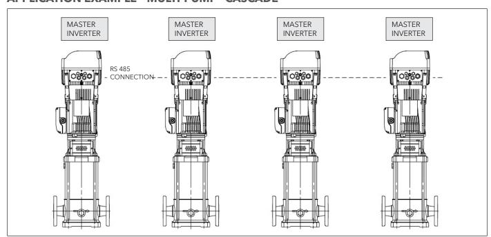
With the "master" version of the Hyrdrovar, it is possible to connect up to 8 Hydrovar controller pumps together in parallel. Complete lead/lag and auto alternation.
