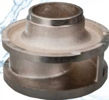
The AK series hydraulic designs utilize either a 2 or 3 vane configuration, depending upon pump size. These impellers also offer a solids passage range from full 3" solids passage on the smaller size pumps and up to a 6" solids passage on the largest pumps for superior non-clog performance. Available hydraulic ranges include 580, 700, 870, 1160 & 1750 RPM motor speeds.
