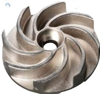
The AV series hydraulics are offered in recessed and semi-recessed vortex impeller designs to provide smooth, clog free operation in the most demanding applications. These enhanced efficiency, multi vane impellers are specifically suited for high solids concentration pumping, and to reliably pass large masses of stringy and fibrous materials. Available hydraulic ranges include 870, 1160, 1750 & 3450 RPM motor speeds.
