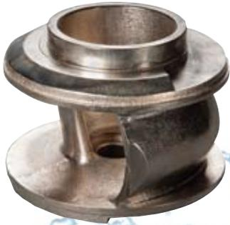
The AMX series hydraulics utilize a single (asymmetrical) concave vane with a smooth, spherical passageway for superior non-clog performance. Enhanced efficiency is achieved without sacrificing solids handling capability (particularly in smaller impeller sizes). The 3" and smaller 4" pumps have a 3" spherical solids passage and the larger 4" and 6" pumps have a 4" spherical solids passage. Available hydraulic ranges include 870, 1160 & 1750 RPM motor speeds.
