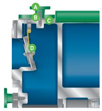
Easily removable knock-off tee handles allow for quick cleaning or replacement of the suction flap valve.
