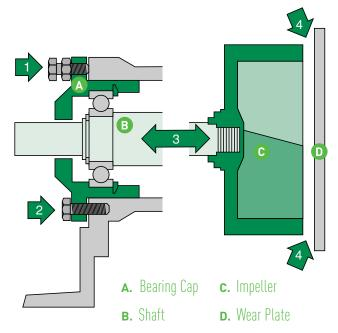
External adjustment allows you to quickly restore original efficiency and performance. External bolts (1 and 2) move the bearing cap, which in turn moves the bearing and shaft assembly (3). This moves the impeller closer to the stationary wear plate for the proper clearance (4) to restore peak performance and save money.
