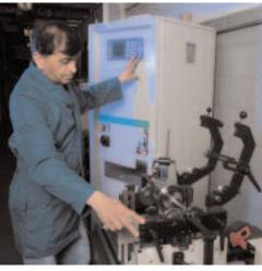
Technician balancing inner magnet for a mag-drive pump: Precision balancing of internal components significantly extends the service life of our products.
