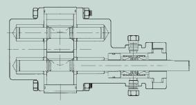
FIG.4 DOUBLE MECHANICAL SEAL
