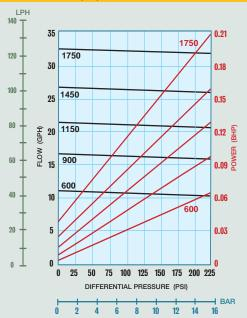
4-SERIES LOW-FLOW GEAR PUMP **MAG-DRIVE**
