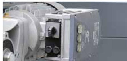
Switches and keys are located directly on the drives and enable direct starting and stopping as well as mode switching.
