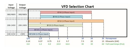
\*\*All applications requiring motors above 3HP, require a VFD or soft start
