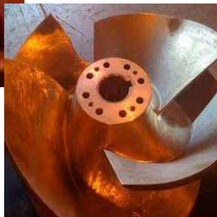
Finished Machined and Balanced Impeller
