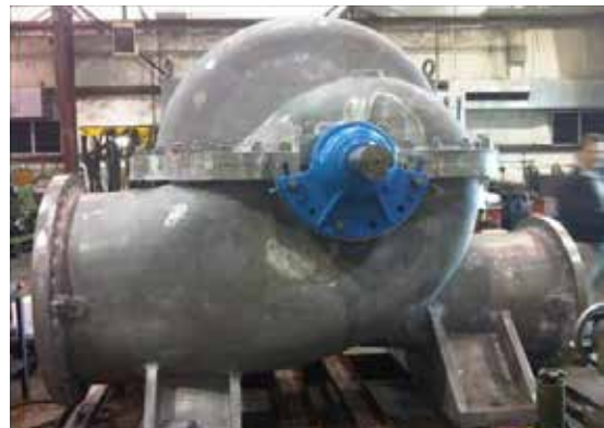
New ProCast casing upgraded from Cast Iron to 316SS
