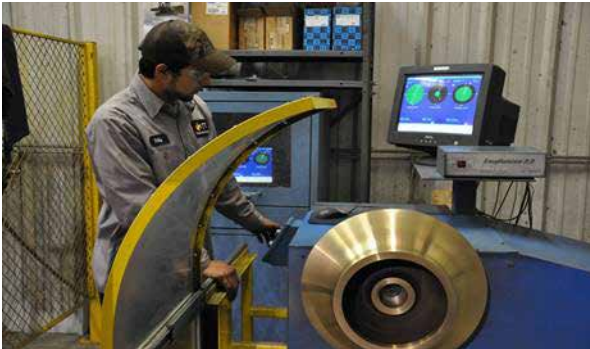
All Impellers & rotating elements dynamically balanced
