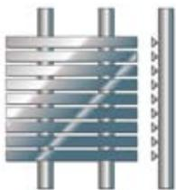
**Wedge Wire (WW)** or slotted, is the most durable of all backwashable media. They are strictly limited to .001" slot or 25 micron as the lowest retention rating. Wedge wire is particularly suited for critical low maintenance applications. As a result of their construction, they are used in many instances where manual cleaning is necessary but might damage other types of media.
