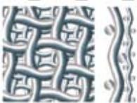
**Poroplate®** filter media is made from layers of stainless steel wire cloth diffusion-bonded together to form a rigid porous metal laminate structure. Poroplate filter media is corrosion resistant, cleanable, and can withstand high temperature applications up to 800°F. Micron ratings from 2 to 150 are available.
