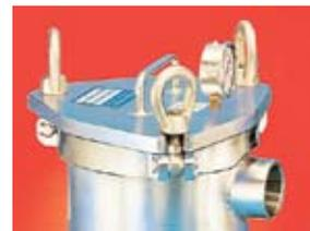
Covers are secured by three eye-bolt assemblies. One of them acts as a hinge, when the cover is opened.
