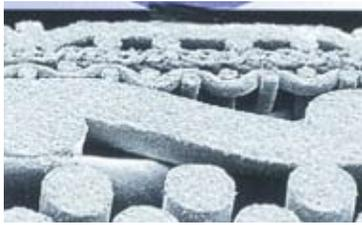
Downstream Support Layers provide reduced differential pressure through open flow channels, as well as higher flow rates and longer filtration cycles. These layers greatly encourage backflushing, keeping the element on line longer.
