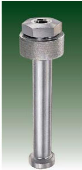
The mini-bag filter is very easy to service too. Just spin the knurled collar loose, push the housing out of line a bit, remove the element, slip a new or clean one in, and you're back in business. The seal is a special, Teflon-encapsulated Viton O-ring. It can be tightened by turning the knurled collar, usually by hand.
