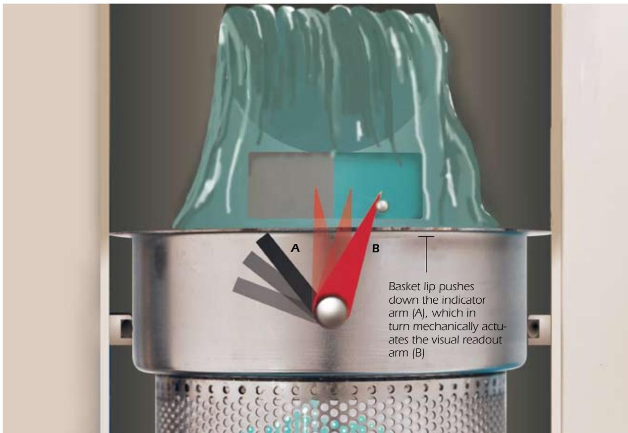
**As Amount Of Trapped Dirt Increases, Pressure Drop Increases, And The Remaining Life Of The Filter Decreases**
