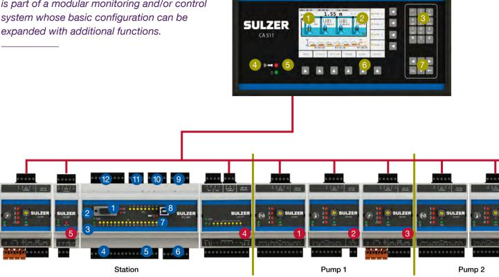
The system shown here provides advanced monitoring of electrical properties, temperature and leakage per pump. The operator panel and the modules described to the right are connected to the PC 441 via the CAN bus interface.
