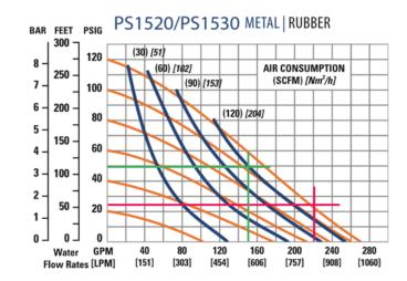
The Husky 3300 can put out 220 GPM vs 25 psi discharge pressure (red). It uses just over 225 SCFM to do it. The Wilden PS1520 can duplicate that performance but uses only 130 SCFM - that's 95 SCFM less - equivalent to more than 20 Hp less energy.
